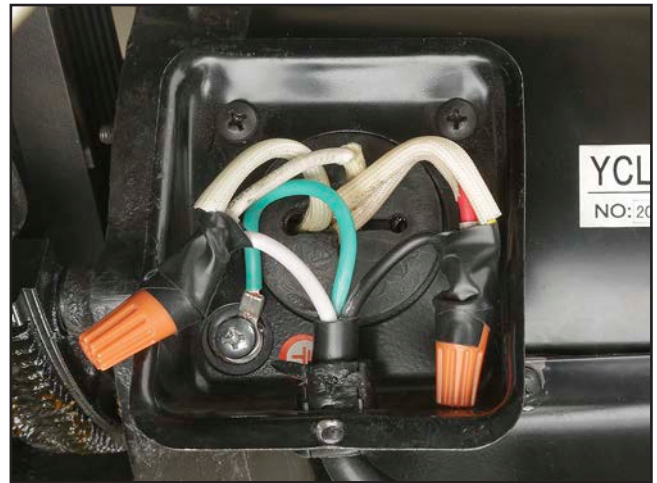
Figure 136. Motor wiring at 120V.
